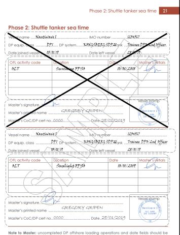
Note to Master: uncompleted DP offshore loading operations and date fields should be crossed out. DP entries cannot be block-signed or completed. DP sea time date entries without the Master's signature or initials will not be counted or validated. Dates should be in dd/mm/yyyy format. Activity codes as per page 12.
